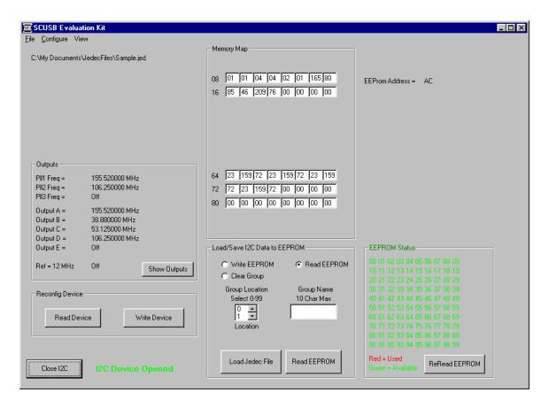
The screen shows us a few things that should be noted. The first thing is that the Output section displays the 2 PLL frequencies we created and the 4 output clocks we also created. Also shown in the center of the screen is the memory map for the JEDEC file.
